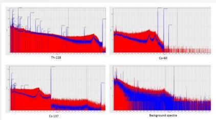
Red spectrum - active shielding is off. Blue spectrum - active shielding is on.
