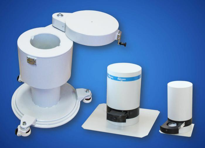
Gamma-, beta- and alphaspectrometer-radiometer TRIO
